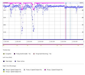
Chart Condition: Chart indicates Supply Water Pressure is way above its 15 PSID Set point but yet it keeps 1 Pump running at 100%. Space Pressure Control – The pump bank is unable to maintain the pressure setpoint. Cause:
